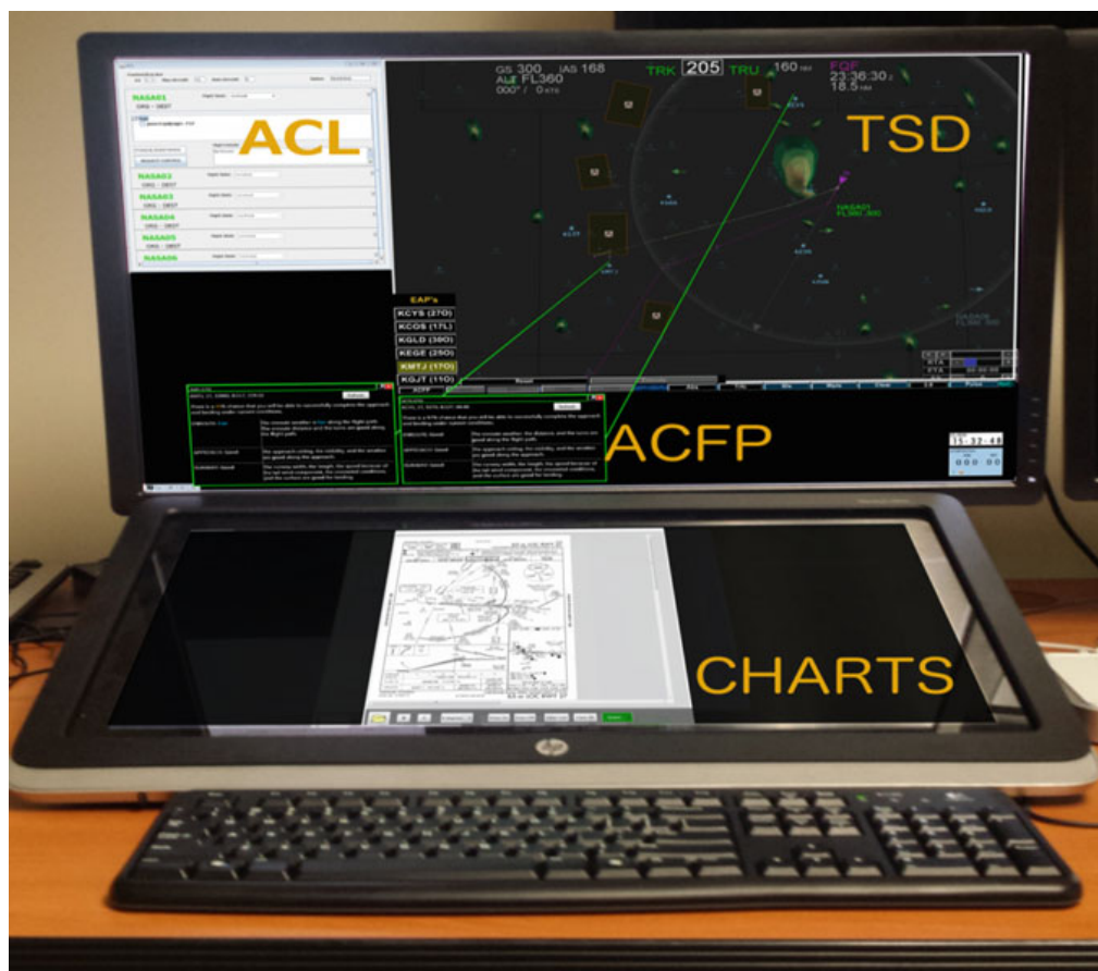
Fig. 1 Example experimental ground station
